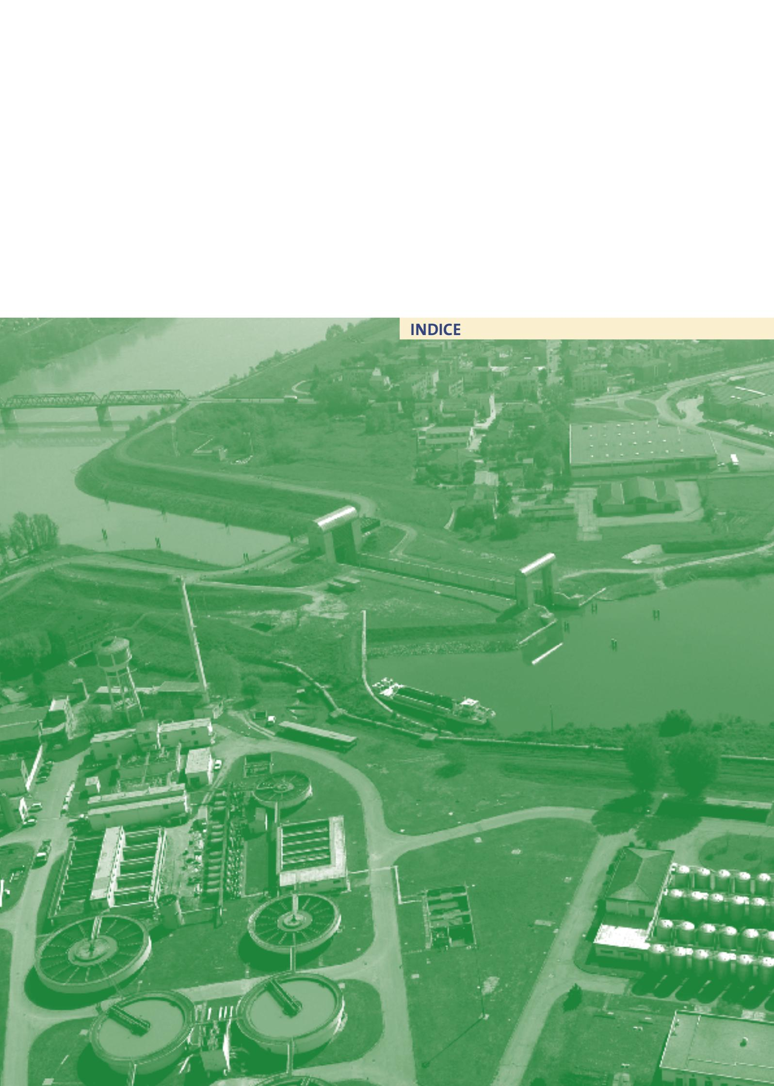
An aerial photograph of a wastewater treatment plant, overlaid with a semi-transparent green filter. The image shows several large circular clarifiers in the foreground, followed by rectangular aeration tanks. A river flows through the facility, with a bridge visible in the upper left. The plant is surrounded by greenery and some industrial buildings.
